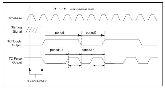
Figure 2-11. Square Wave Timing
